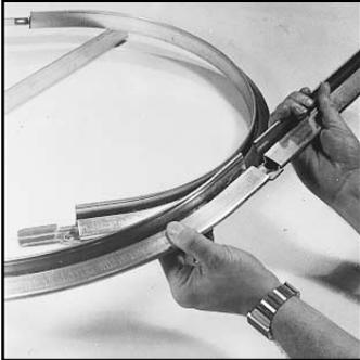
4. Slide the two "straight" oval angle pieces onto the connector pieces already inserted into the curved Ovalmate sections. Make sure the connector pieces are seated completely into the Straight and Endset. This will be known when both flange ends butt up to the notched section of the connector piece that you install the bolt in. See picture under step 9.
