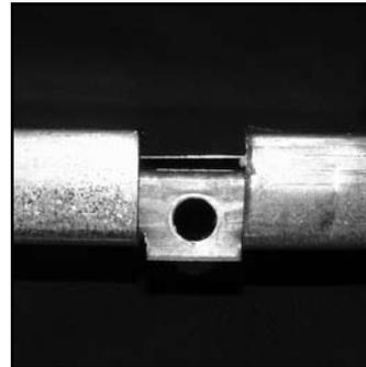
9. The duct must be seated all the way into the Ovalmate angle in order to penetrate the integral sealant and avoid air leaks. Double check to make sure that the duct edge protrudes past the downset of each Ovalmate connector piece.
